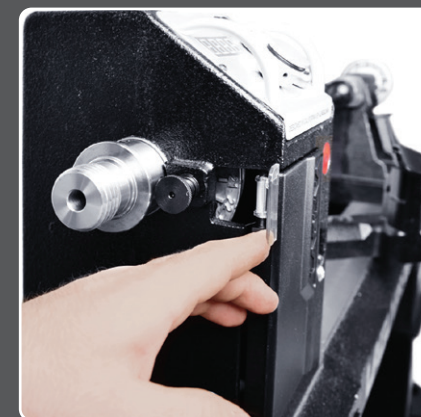
Spindle indexing in 24 points
